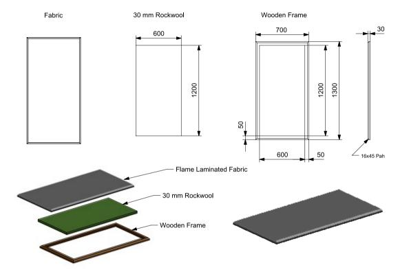
Acoustic panel made of rockwool and coated acoustic fabric, for installation we developed unseen screws system for easy installition to the wall without necessarily need of a metal frame in the wall.
